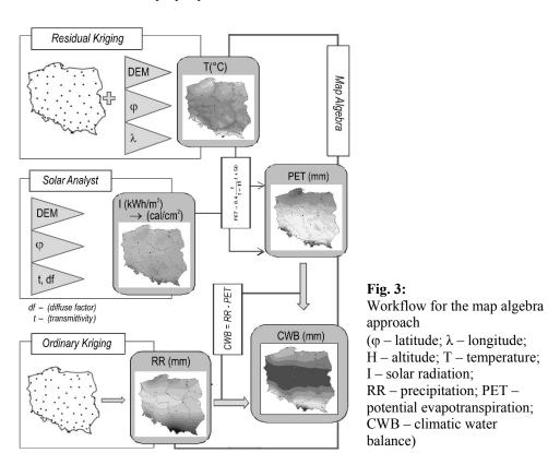
All the layers created were used as an input data to potential evapotranspiration model by Turc's formula (air temperature together with solar radiation map) and further on with precipitation map to calculate climatic water balance for the area of Poland according to map algebra methodology (figure 3).
