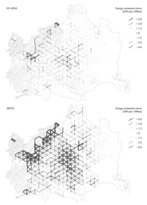
Fig. 3: Spatial distribution of energy estimation errors based on EU-DEM and SRTM3.0
