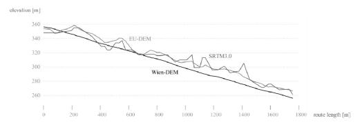
**Fig. 4:** Route profiles of a sample route, energy estimate difference: +12.96kWh (EU-DEM) and +31.94kWh (SRTM3.0)
