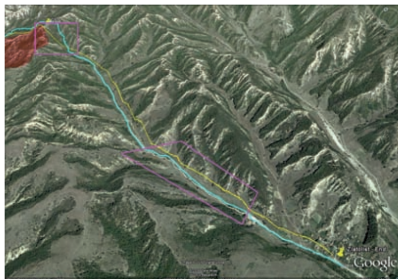
Fig. 35: Differences between the existing route (in turquoise) and the calculated “least-cost path” (in yellow) on the southern versant; © 2009 Google, © 2010 Tele Atlas, Image © 2010 DigitalGlobe, © 2010 Basarsoft; KML layer by Juilson J. Jubanski
