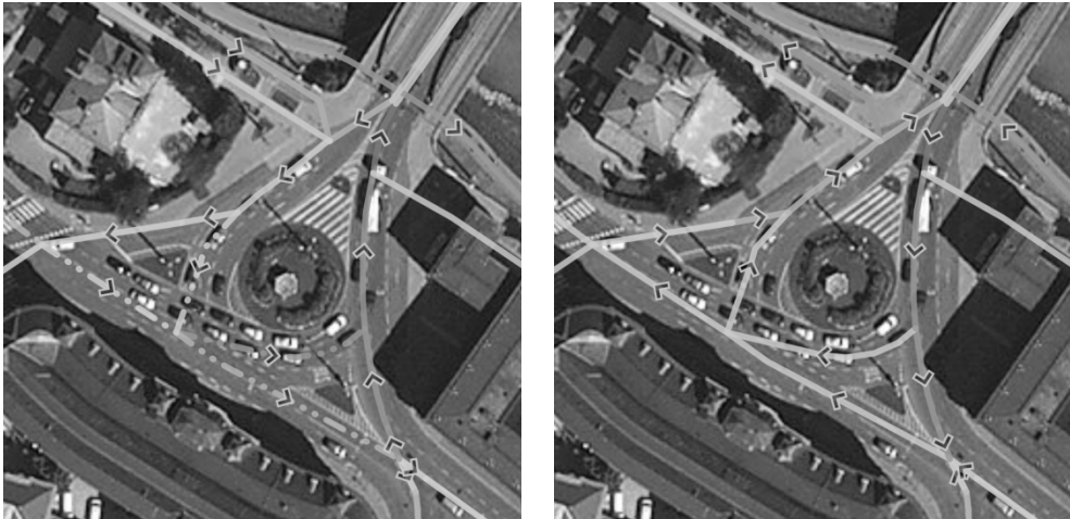
Fig. 2: Intersection rendered for different directions (road segments are colored according to the index values; one-ways have a different line symbol along the digitized direction; one-ways are restricted against the digitized direction)
