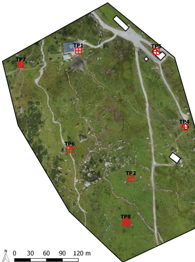
Figure 11: GCPs used for georeferencing at the Austrian study site (Tie Point – TP1-8); distribution within the RPAS-AOI (left); detail of TP1 & TP7 location (right) - both against the snow-free RPAS OP.
