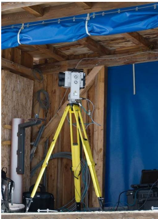
Figure 12: Riegl LPM-321 (left) and LPM 98-2k (right) in operation for snow depth monitoring at the Austrian study site on 11 Feb 2015 and 13 Feb 2015, respectively.
