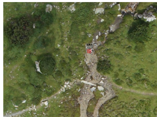
Figure 11: GCPs used for georeferencing at the Austrian study site (Tie Point – TP1-8); distribution within the RPAS-AOI (left); detail of TP1 & TP7 location (right) - both against the snow-free RPAS OP.
