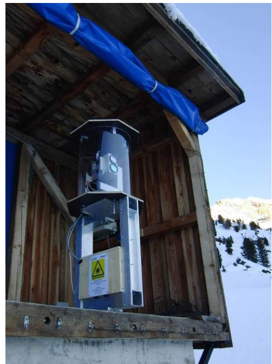
Figure 12: Riegl LPM-321 (left) and LPM 98-2k (right) in operation for snow depth monitoring at the Austrian study site on 11 Feb 2015 and 13 Feb 2015, respectively.
