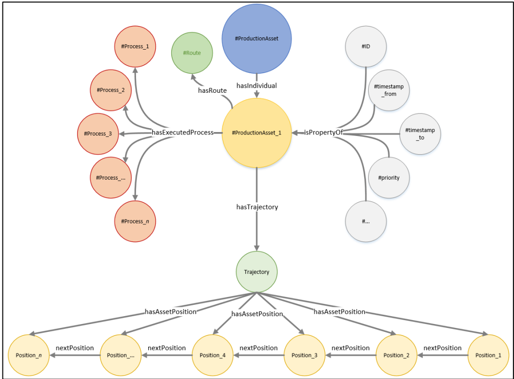
Figure 3: Digital representation of production assets and their linked datasets. Each individual production asset (in yellow) has a unique trajectory (in light green), where the points (in light yellow) are stored in a temporal sequence, denoted with the typed link 'nextPosition'. A unique Route is part of each production asset (in green). Each production asset has properties, which are marked in grey. Executed Processes are marked in light red.
