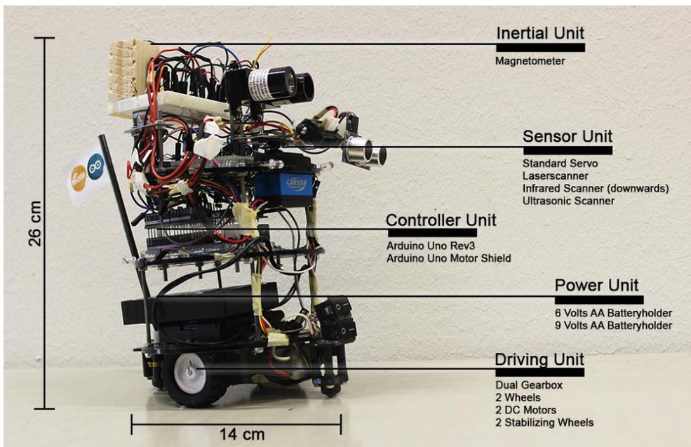
**Figure 2:** Configuration and dimensions of the SLAM robot.
