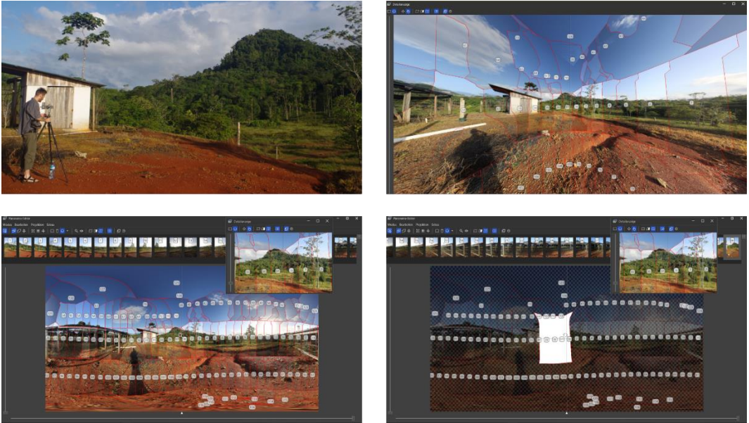
Figure 1: Transformation and distortion of single photographs taken by DSLR cameras in the creation of a spherical virtual replica using PTGui. From top left to bottom right: generation of photographic source files; merged images in spherical simulation; mosaic display of source files; distortion of source files within the panorama
