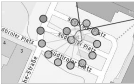
Figure 4: Spiral spreading of overlapping points when the maximum zoom level is reached
